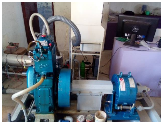
Kirloskar TV1 Engine experimental setup.
